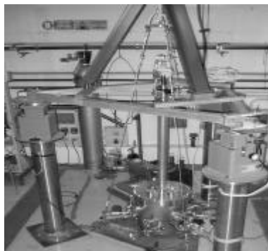
Figure 5: The torsion pendulum based test bench for the sensor. The picture shows (a) the vibration-isolation pods. (b)The torsion suspension of the apparatus. (c) The high vacuum chamber. (d) The micro-positioning system to center the electrode housing relative to the test-mass
